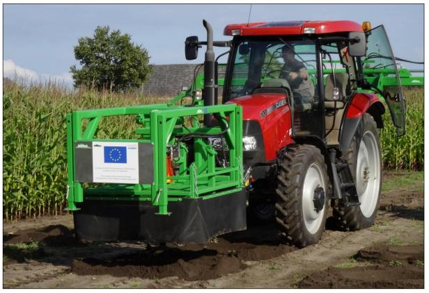
The direct capillary drill consists of a 3-point frame with support wheels, in height adaptable. A hydraulic driven drill column is installed in the frame. Lowering and lifting of the drill is done by the lift arms of the tractor. The required hydraulics are supplied by the tractor (not included). It can be installed on the front or rear of a tractor.
