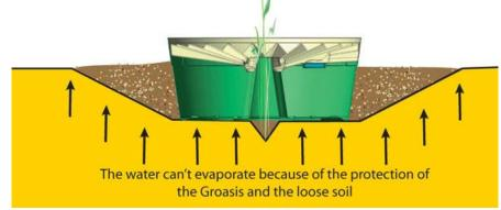
The Groasis Waterboxx is a Popular Science awardwinning invention that was inspired by how seeds grow in desert regions of the world. Using a drip irrigation system combined with a self-refilling container, water needed to grow the grapes does not evaporate away.
