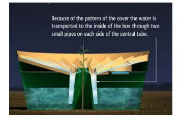
Every night new condensation is created on the surface grooves runs down into the reservoir, and also any rain is captured in the tank too, replacing the dripped out water below, so once filled, no new water is needed to keep the drip irrigation going.
