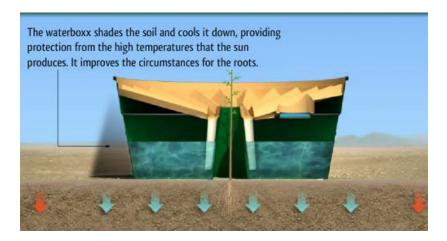
Essentially, the way it works is it is a self-refilling container for water for drip irrigation. Due to the enclosed container design, the water won't evaporate away. You only need to fill the outer bucket tank half full with water once.
